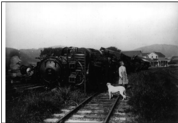
Figure 9-3. A famous historic photograph taken by an engineer of a derailed train that tipped over at the Point Reyes Station during the 1906 earthquake (image from Jordan, 1907). The narrow gauge train was stopped at the station on a section of track that ran roughly parallel to the fault several hundred meters east of the rupture. Based on the engineer's description of the rocking motion that fell the locomotive, Anooshehpour and others (1999) calculated the earthquake motion created ground acceleration that was in the range of 0.7 to 1.1g.
