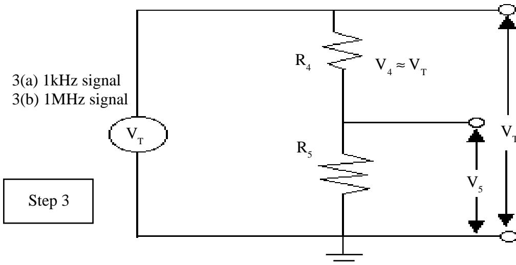
**Step 3(b)** Repeat 3(a) using a frequency greater than 1MHz.
