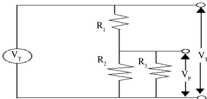
A second limitation of the divider is more subtle. For AC signals, the voltage divider action is not only due to resistance, but must also include any reactance which may be due to capacitance. This can be particularly troublesome at high frequencies and at large ratios. The effects of this AC limitation is demonstrated in step 3.
